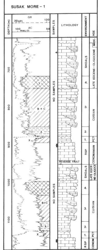
Fig. 6 Sequence of Palaeogene carbonates in the deep well Susak More-1. For legend see Fig. 2.
