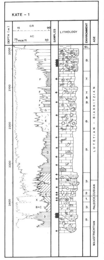
Fig. 3 Sequence of Palaeogene carbonates in the deep well Kate-1. For legend see Fig. 2.
