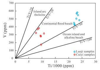
Figure 8. Classification diagram of Ti/1000 vs. V for basaltic magma (after SHER-VAIS, 1982).
