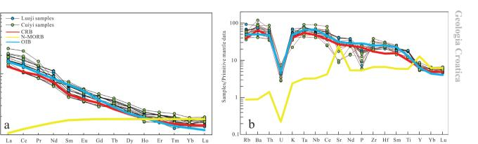
Figure 5. (a) Chondrite-normalized REE distribution pattern and (b) primitive mantle-normalized spider diagram for the samples (after SUN and MCDONOUGH, 1989).
