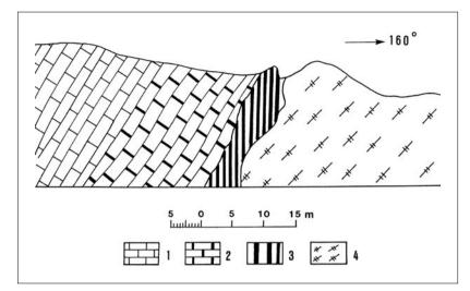
Fig. 3 Profile through the contact of gabbrodiorite and platy crinoidal limestone with a magnetite ore body (after ČELEBIĆ, 1967). Legend: 1) platy crinoidal limestones; 2) contact-metamorphic limestones/marbles; 3) scarn; 4) gabbro diorite.
