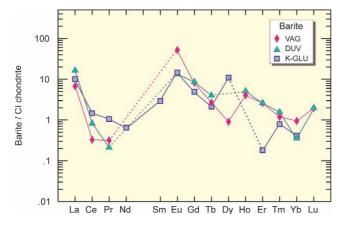
**Figure 3:** Plot of CI chondrite-normalized REE abundances (SUN & McDONOUGH, 1989) of barites (VAG, DUV and K-GLU) from the Duboki Vagan and Glumac barite deposits. Data for the K-GLU sample are from JURKOVIĆ et al. (2010).
